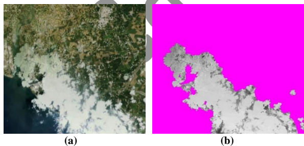
Fig.12. Cloud region segmentation by Grab Cut: (a) original image; (b) result image;
